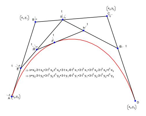
Point E is proportion t along the line AB. Point F is proportion t along BC. Point G is proportion t along CD. Point H is proportion t along EF. Point I is proportion t along FG. Point J is proportion t along HI. The spline curve is the locus as t runs from 0 to 1.
